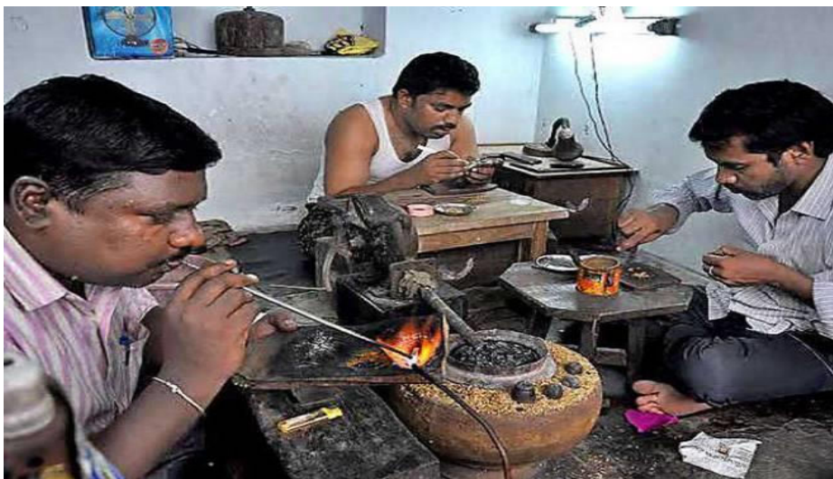
Plate 25.6: Goldsmiths melting the gold in a crucible.
